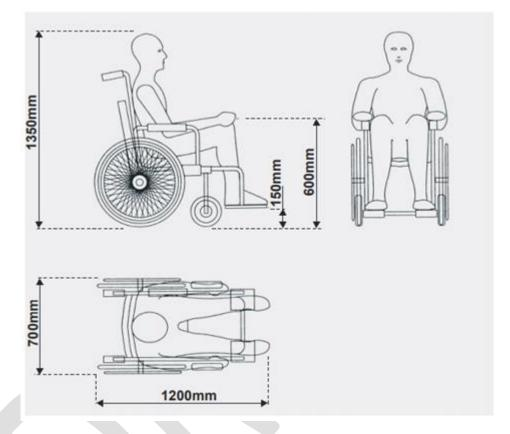
The reference wheelchair has: a total length of 1200mm including extra-long footplates total width of 700mm sitting height (from ground to top of head) of 1350mm. The reference wheelchair is bigger than most wheelchairs to ensure that enough room is provided for most wheelchair users.
